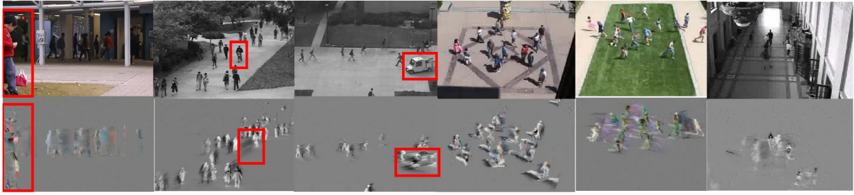
Fig. 6. RGB input vs. Output of Motion Fusion: the motion fusion block shows advantages of removing the irrelevant background and focusing on the abnormal objects. Note that, in the second example, it is hard to visually detect the bicycle (anomaly) from the front view, however our motion fusion block is able to visually keep the moving pattern information with a black tail in a single compressed image.
