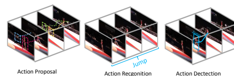
Fig. 1. Conceptual illustration of the difference among action proposal, action recognition, and action detection. Action proposal tries to extract all possible human actions which are highlighted using dash-lines. Action recognition aims to classify the whole video into specific categories, e.g., 'Jump'. Action detection aims at detecting when and where a specific action appears (highlighted using solid-lines).
