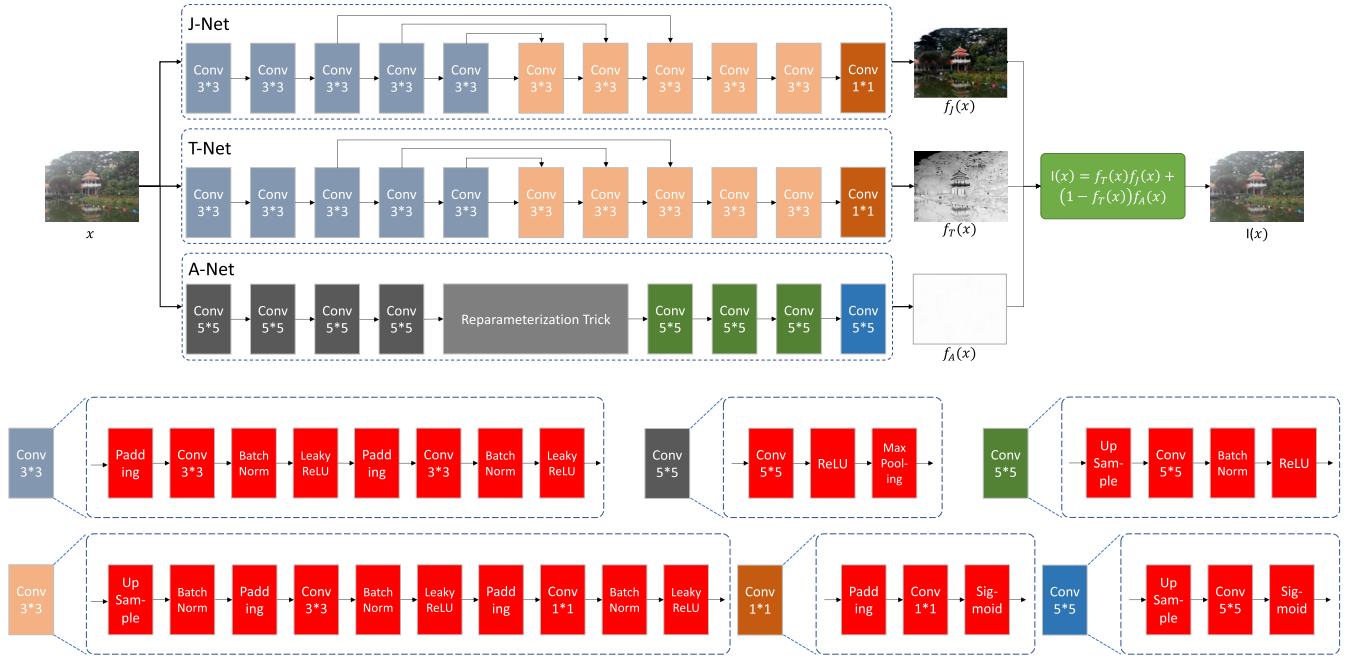
Fig. 2. The framework of our proposed ZID. ZID includes three parts: clean image estimation network (J-Net), the transmission map estimation network (T-Net), and the atmospheric light estimation network (A-Net).
