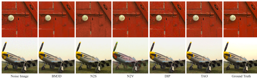
Figure 5. Qualitative results on image denoising, from which one could observe that existing methods excessively denoising resulting in smoothing and/or artifacting of the images. In contrast, our method obtains clearer and sharper results which are closer to ground truths.
