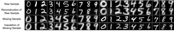
Fig. 6. The imputation of the unobserved samples with the missing rate of 100%. The raw samples are the inputs x_i^{(v_2)} drawn from MNIST (left half) and USPS (right half). The unobserved samples are x_i^{(v_1)} which is invisible to our model. The reconstructions and imputations are the \hat{x}_i^{(v_2)} = g(f(x_i^{(v_2)})) and \hat{x}_i^{(v_1)} in Algorithm 1 line 16 in Supplementary respectively.
